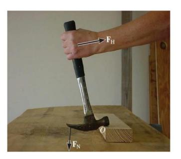
Carpenters often use a hammer in this way to pull a stubborn nail. Through what sort of action does the force  $F_H$  at the handle pull the nail? How can you mathematically model the effect of force  $F_H$  at point O?
